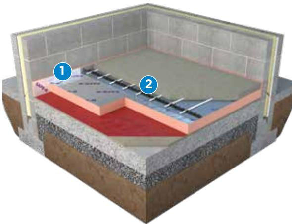
1. Good detailing at the wall/floor junction is essential to reduce thermal bridging. By placing an upstand of Unilin Perimeter strip (SR/STR) 25mm thick around the external and internal wall/floor junctions, an improved detail is created.
